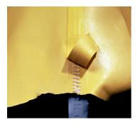
**TRELLCHEM EVO/VPS SEAM** Stiched with aramide thread for superior strength and durability. Taped with a rubber strip on the outside and a barrier laminate strip welded to the inside. This provides a continuous barrier layer across the seam.
